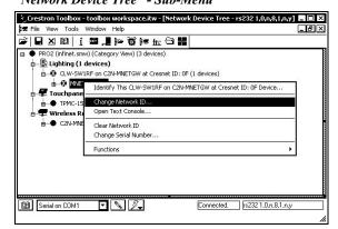
**NOTE:** Any infiNET switch in the Network Device Tree can be identified using Crestron Toolbox. Right-click a device in the Network Device Tree and select "**Identify this...**". The LED on the switch will flash HIGH. Press a button on the switch to identify the device.
