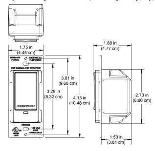
The -SW1RF, -SW4RF, -SWS1RF, -SWS4RF, and -SLVS1RF mount in a standard wallbox and are covered using a decorative faceplate (not included). All line voltage connections are made at the rear of the switch.
