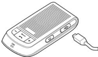
Figure: 2 Battery Charging
