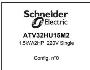
Display after the drive has been powered up for the first time.
