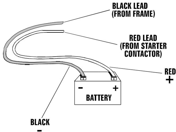
Figure 6.3 – Battery Cable Connections
