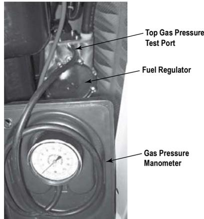
**Figure 5.5 — Checking Pressure with Manometer**
