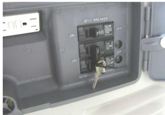
Figure 2.3 — Circuit Breaker Box and Keys (as shipped)
