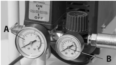
Tank pressure gauge (A) & Outlet pressure gauge (B)
