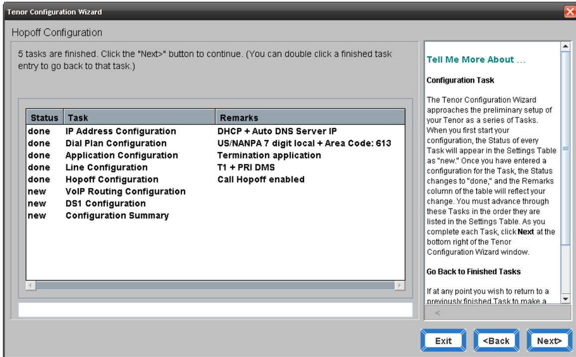
22. On the VoIP Routing Configuration screen, for integration with the UC server, choose **SIP only**. Select **Next>** to continue.
