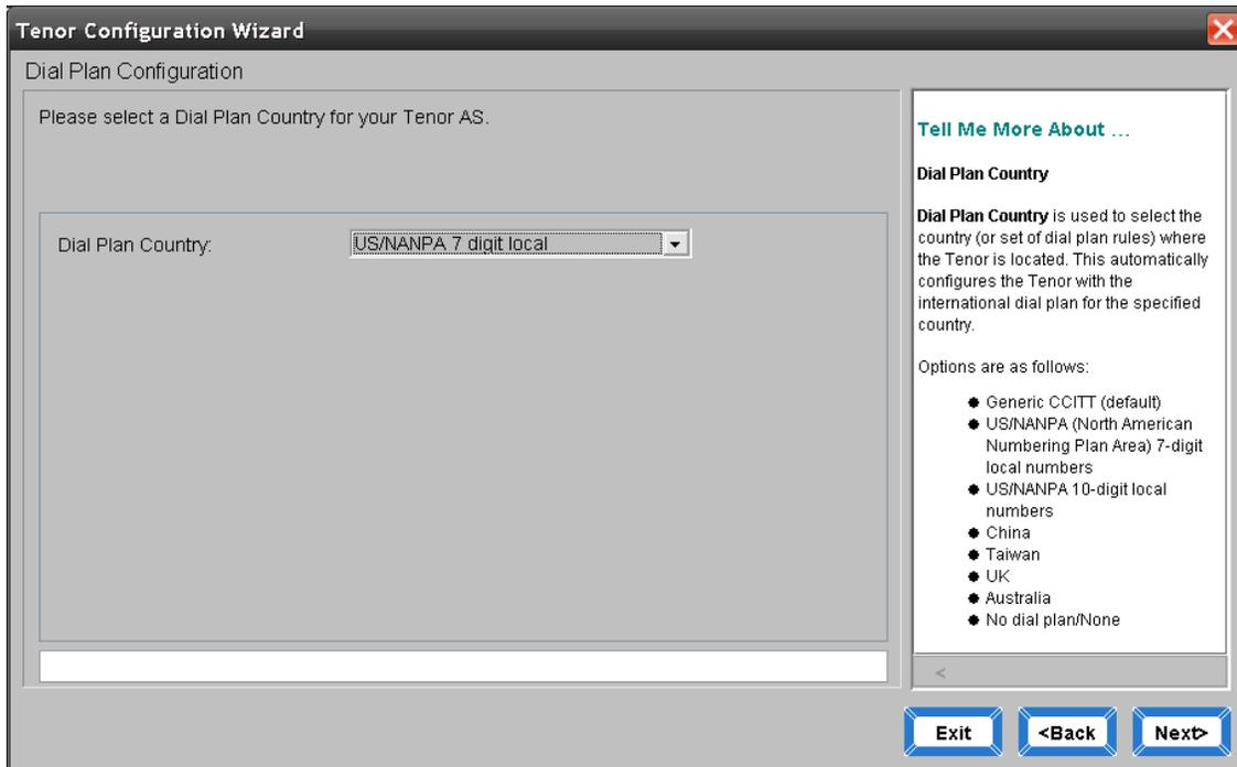
8. On the next Dial Plan Configuration screen, enter your local area code, which the Tenor uses to correctly route calls through the PSTN. Select **Next>** to continue.
