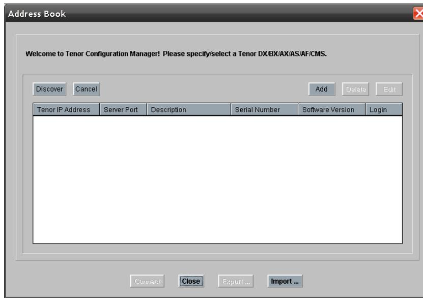
1. In most cases, by selecting **Discover** the program automatically detects the gateway. Select **Connect**. If the program does not detect the gateway, you must select **Add** and manually enter the IP address of the Quintum gateway.
