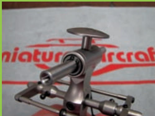
Headblock with feathering spindle fitted, note the circlip is fitted with sharp side facing the end of the spindle
