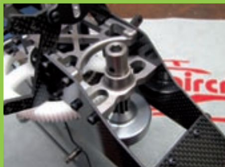
Clutch bell and start cone fitted
