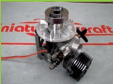
Completed engine fan and clutch assembly
