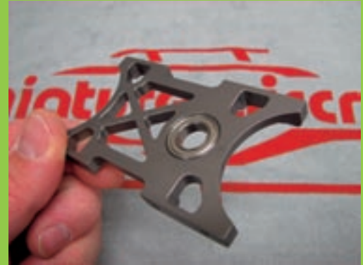
The bearing blocks have been cut out and the edges rounded to reduce their overall weight
