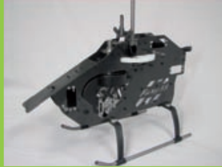
Left side of completed frame assembly
