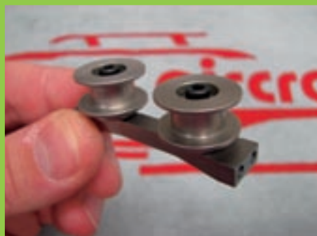
Machined tail belt tension pulley assembly
