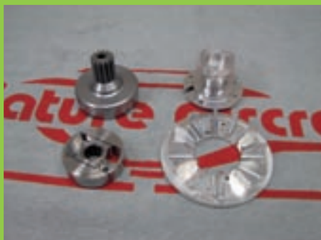
Clutch and clutch bell, fan and fan hub parts
