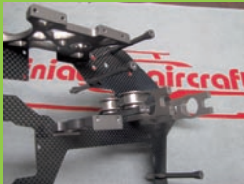
The main chassis for the helicopter is a typical two carbon frame assembly held together with aluminium spacers
