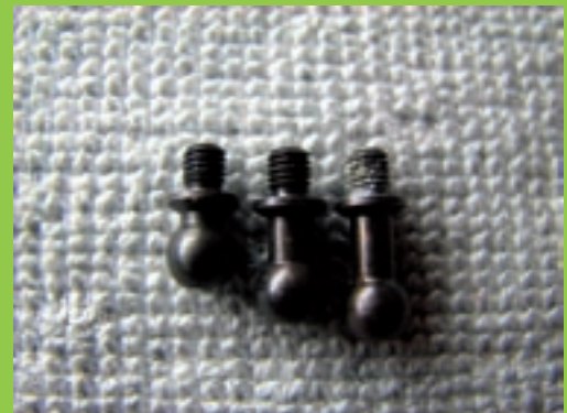
Swashplate balls showing the similar inner balls
