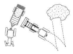
To increase loading efficiency. Minimize angle of turn and length to run between pile and spreader.
