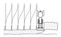
Leave material, which drifts over the bucket sides for final cleanup.
