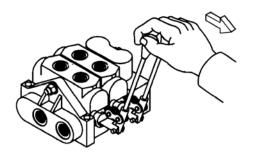
Work both levers back to direct pressure to both cylinders.
