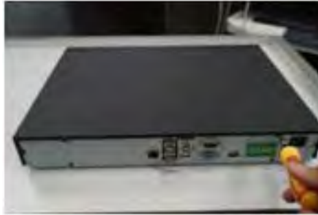
Figure 2-4 Removing the NVR Cover
