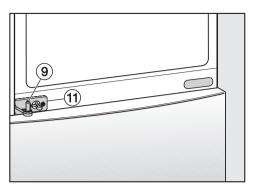
■ Fit hinge pin ⑨ into middle hinge plate ⑪ in the lower door.
