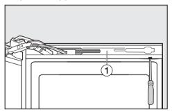
■ Prise open ① from the soft-close mechanism by inserting a flat-bladed screwdriver into the gap from above and easing it off bit by bit.
