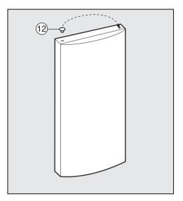
■ Remove cap <sup>12</sup> from the bush in the door and refit on the opposite side.
