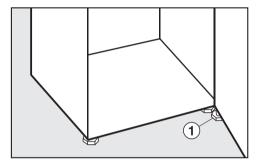
■ Also unscrew support ① from the hinge plate, to level the appliance door.
