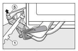
■ Push hinge pin ⑤ up and out from underneath.
