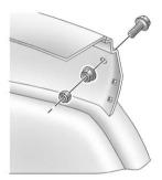
A 10 mm ground stud can be found in the trunk on the passenger side of the vehicle. The stud is located above the trunk auxiliary junction block. See "Trunk Auxiliary Battery Power Junction Block" that follows for more information on location.
