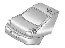
About 240 cm (95 in) of RG58 coaxial radio antenna cable is run from the roof panel just rear of the center dome lamp and coiled in the trunk to reach either corner. The cable permits the connection of customer-installed communication equipment.
