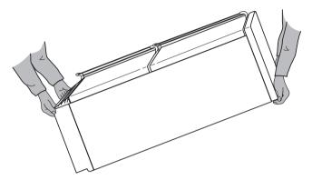
2. In order to push the appliance into its final position, press carefully at the top of the door and tip the appliance back slightly. The weight is thus transferred to the back wheels and the appliance can be easily pushed.
