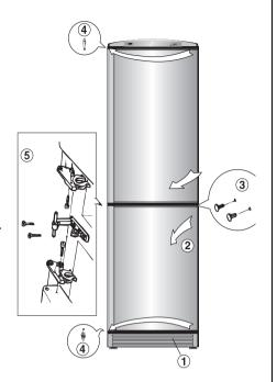
After changing the door hinges, check that the magnetic seals on the doors fit perfectly against the housing and that the interior lighting goes off when the door is closed.
