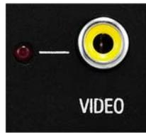
**FIG. 25** Composite output
