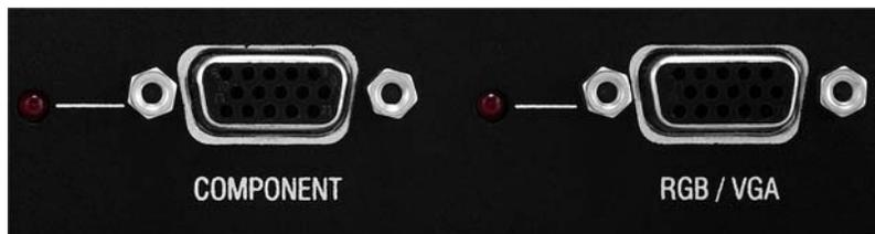
**FIG. 26** HD-15 Output connectors
