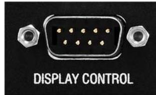
**FIG. 20** DISPLAY CONTROL connector
