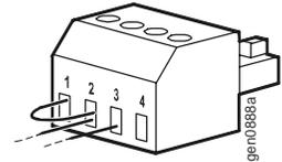
**Note:** The power for operating the EPO circuit is sourced from pin 1. This is an isolated 24 V which can source only a few milliamperes.
