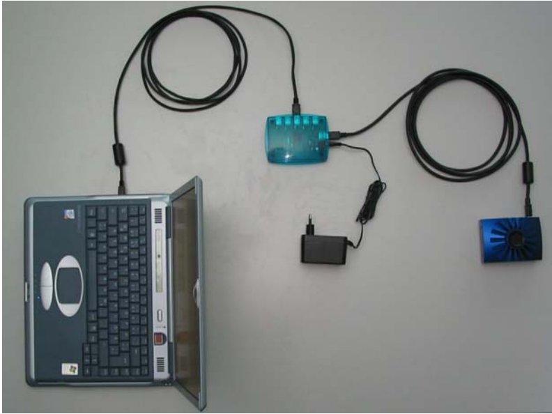
Connecting the AxioCam MRc5 to the onboard FireWire interface of the notebook
