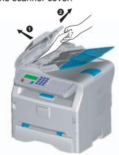
**2** Remove the jammed paper without tearing it. The following message appears:
