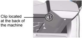
2 Lift the scanner to access the analysis glass.
