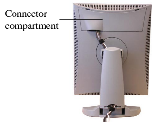
Signal cables routed under foot cover and bound by velcro strips
