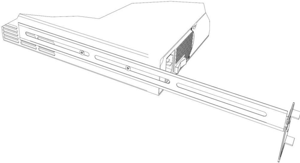
2. Attach the appliance rails to the appliance using three appliance rail screws.
