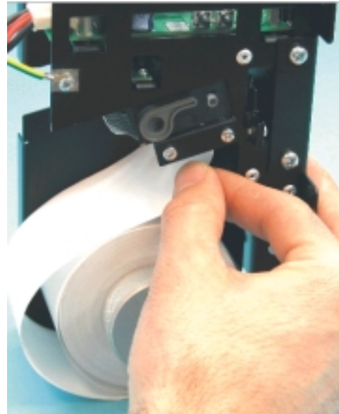
Fig.3.1- Automatic paper load.
