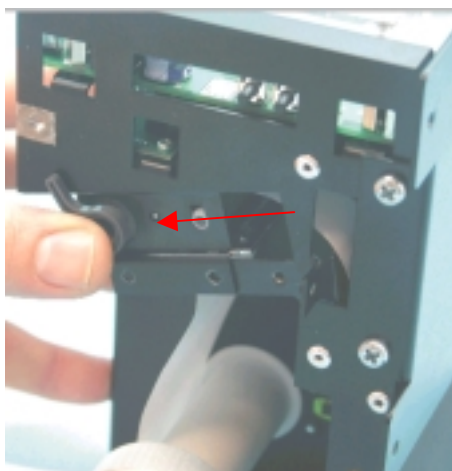
Fig. 3.9- Paper jam recovery.
