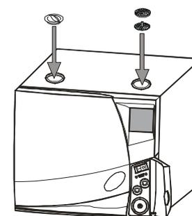
**If the sterilizer is not used for more than 3 days, both water tanks must be completely drained in order to avoid alga growth or any other deposits.**
