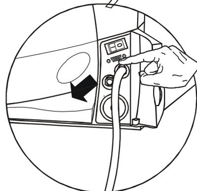
**If the sterilizer is not used for more than 3 days, both water tanks must be completely drained in order to avoid alga growth or any other deposits.**
