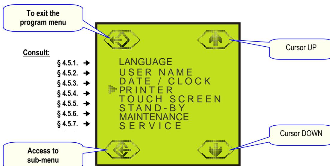
... Place the cursor ">" in front of the desired sub-menu using the "UP" and "DOWN" keys.
