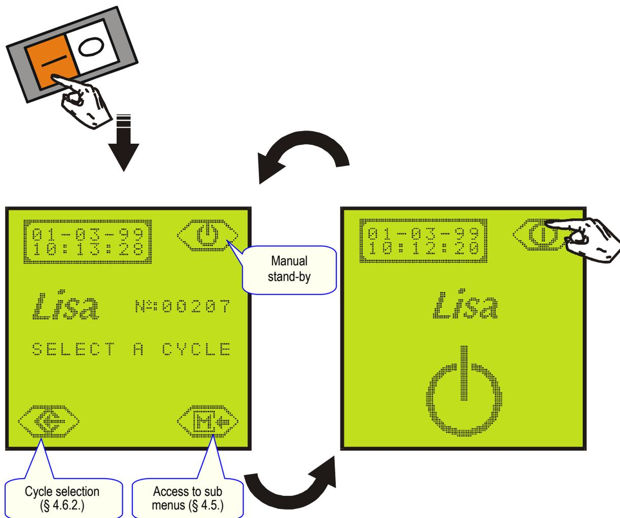
If the sterilizer is not used for a certain period of time, it will automatically go into stand-by mode. Stand-by mode time is programmable (§ 4.5.6.).
