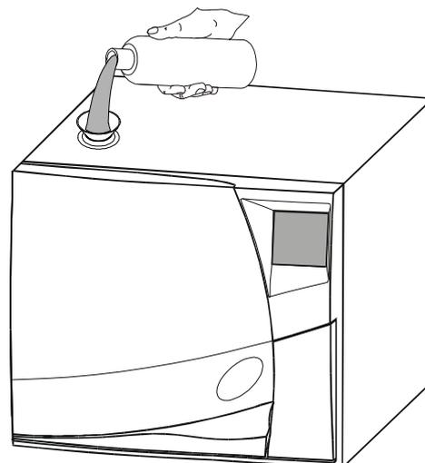
...Fill the tank with approx. 3 litres on MB17 (or 4 litres on MB22) of water...
