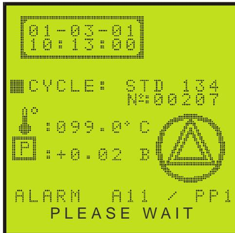
Press the "OK" icon at the end of the re-initialisation phase to confirm the reading of the alarm.
