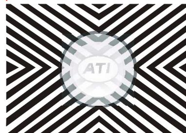
The result is also incorrect, if the indicator is grey or silver (over-exposure, i.e. excessive temperature).
