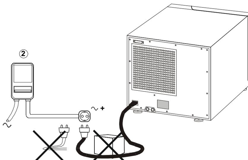
Plug in the mains cable to the back of the sterilizer.
