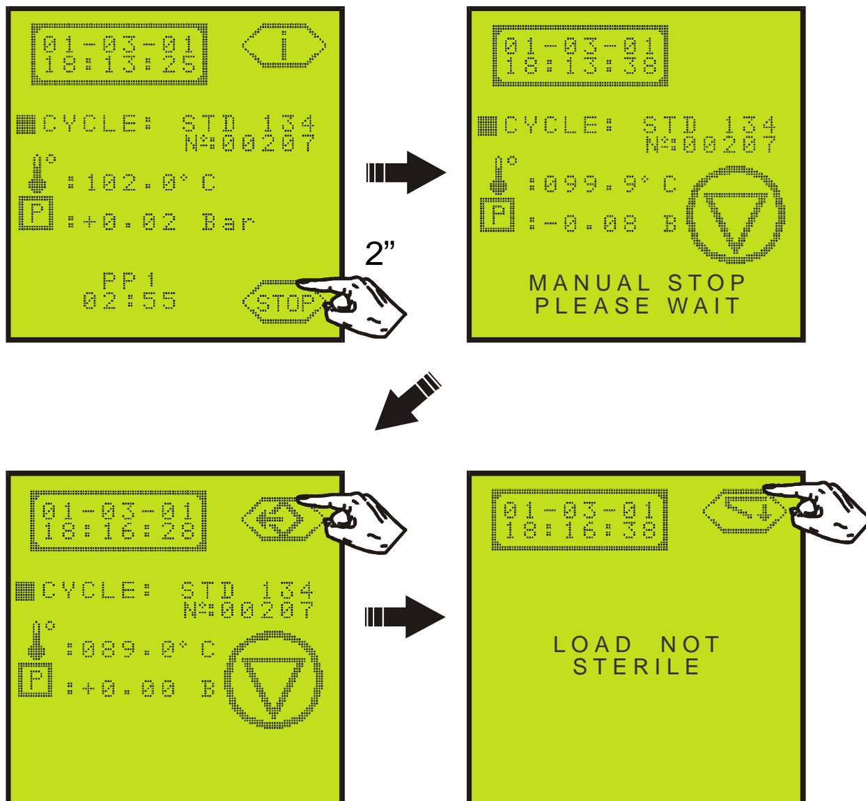
...This is followed by a phase of approximately 2 minutes, required to reinitialise the system and return the chamber to atmospheric pressure.
