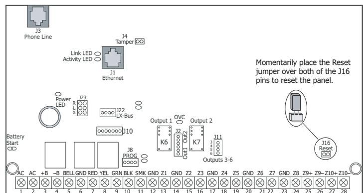
**Figure 9: XR100 Series Panel Showing the Reset Jumper**
