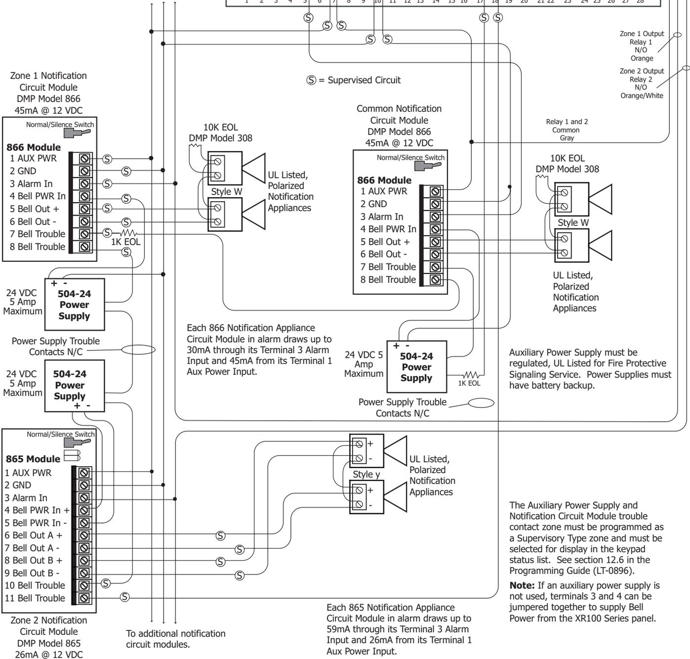
Auxiliary Power Supply must be regulated, UL Listed for Fire Protective Signaling Service. Power Supplies must have battery backup.
