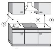
There must be a minimum safety distance of at least 30" (760 mm), ②, between the top of the cooktop and any cabinet above it. The overhead cabinet depth, ③, if unprotected, must not exceed 13" (330 mm). The minimum distance of combustible surfaces located above and to the sides of the cooktop, ④, is 18" (457 mm).
