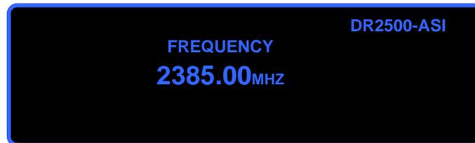
Press again the button "OK" for 2-3 seconds to be able to change the frequency range. After pressing "OK" for the second time the first digit is highlighted and the display looks like in *figure 7*. Press the "UP" control button to increase the digit and the "DOWN" to decrease, to move to the second digit press the "RIGHT" control button or Press the "LEFT" to come back to the previous digit.
