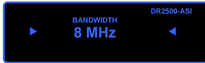
Now it is possible to select with the UP/DOWN button the bandwidth of the transmitted signal you want to receive. To confirm the selected preset press the "OK" button and after that it will appear "UPDATING DEVICE".
