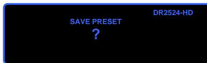
This menu gives the user the possibility to save a frequency under the current preset. Now press again the button "OK" for 2-3 seconds and you will have the choice between "YES" (to save frequency to current preset) and press the OK button.
