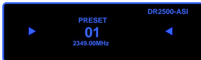
Now it is possible to select with the UP/DOWN button 1 of 26 presets. To confirm the selected preset press the "OK" button and after that it will appear "UPDATING DEVICE".
