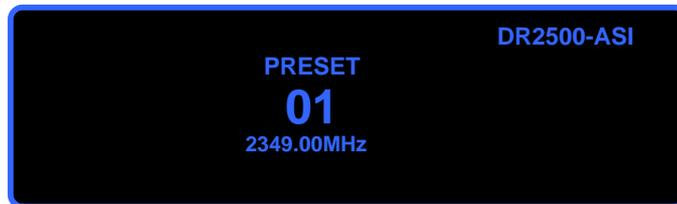
To change the preset number press again the button "OK" for 2-3 seconds to be able to change the preset. Two small triangle will show that the change mode is activated.
