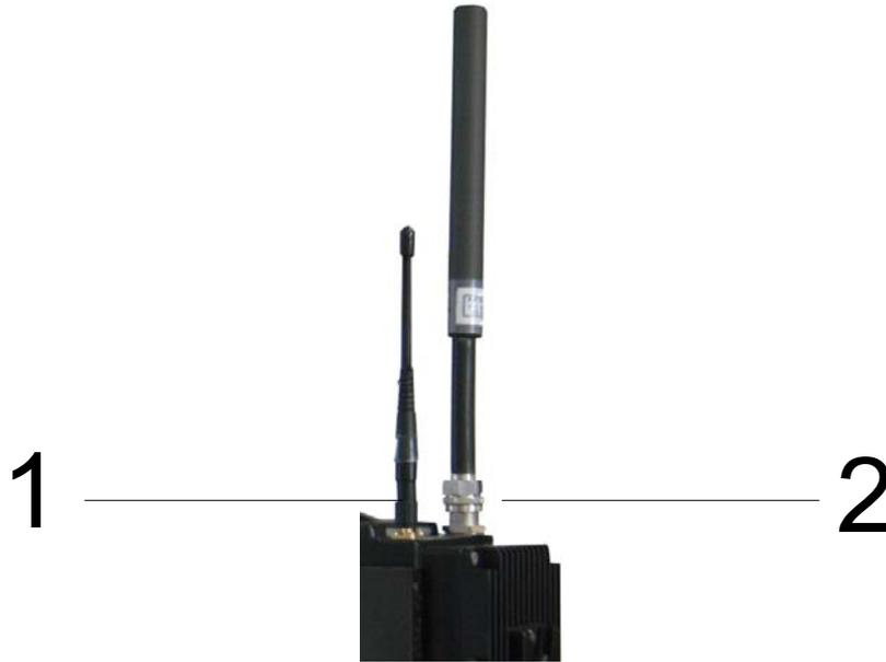
Figure 2: Antenna Sockets
