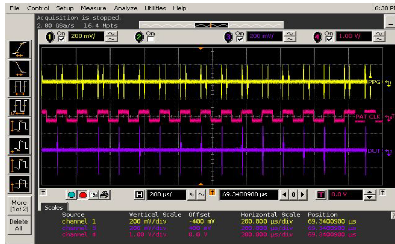
Figure - 3 Example OOB-06 test stimulus and PUT response for out-of-range COMWAKE (Test stimulus top, yellow. PUT response bottom, purple.)
