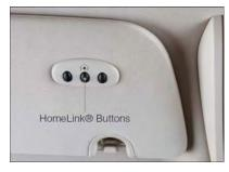
Erase all channels before you begin programming. To erase the channels, place the ignition switch into the ON/RUN position, then press and hold the two outside HomeLink® buttons (I and III) for up to 20 seconds or until the red indicator flashes.
