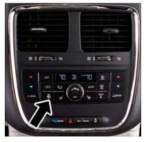
**Heated Steering Wheel Switch Location**
