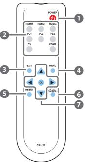
OK & ▲ ▼ ◀►: Press OK to confirm the selection or press the arrow buttons to scrolled in the OSD selections.
