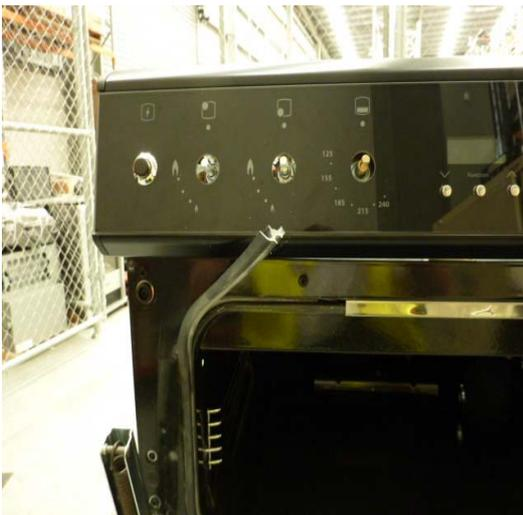
THE DOOR SEAL IS REMOVED BY JUST PULLING IT IS SECURED IN THE GAP BETWEEN THE CAVITY AND FRONFRAME AND REQUIRES NO OTHER FIXING
