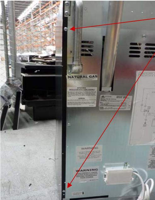
REMOVE 2X SCREWS AT REAR OF APPLIANCE
