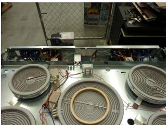
LIFT THE BASE UNIT AND REST IT ON THE REAR OF THE APPLIANCE TO GAIN ACCESS TO THE THERMOSTATS AND REGULATORS
