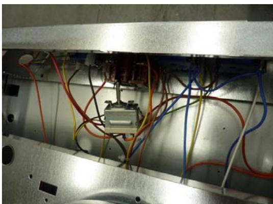
THE THERMOSTATS CAN NOW BE REMOVED BY PULLING OUT OF THE SWITCHPACK
