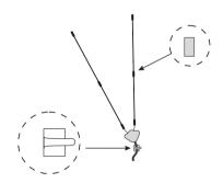
Connection of the antenna to the tuner box
