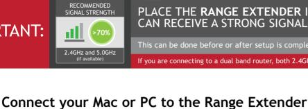
CAN RECEIVE A STRONG SIGNAL FROM YOUR WIRELESS ROUTER This can be done before or after setup is complete. The Range Extender will save your settings. If you are connecting to a dual band router, both 2.4GHz and 5.0GHz connections should be greater than 70%.
