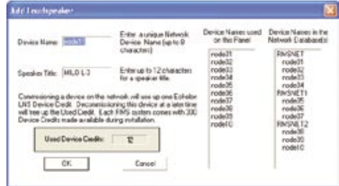
Figure 4.3. The Used Device Credits field keeps track of the number of “credits” (or loudspeakers) on your network.
