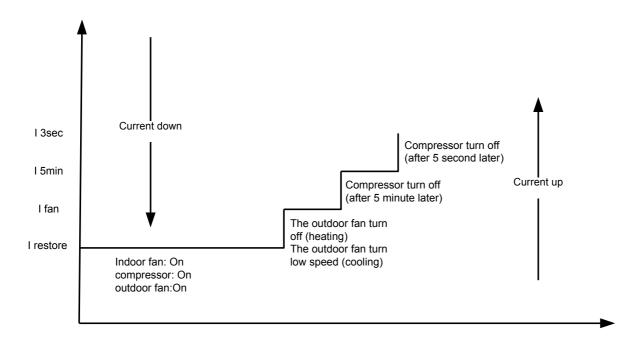
If compressor turns off for continuously 4 times due to current protection in 5 minutes from Compressor On, the unit stops and LED displays failure information and can't returns to normal operation automatically.
