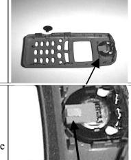
3. Place the keypad mat in the upper housing section.
