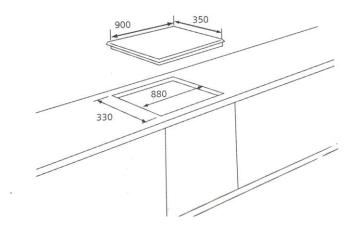
The diagram illustrates the cutting size and additional shaping required for the built-in cave installation. It is always crucial for you to measure the actual ceramic hob dimension before making any cuts.
