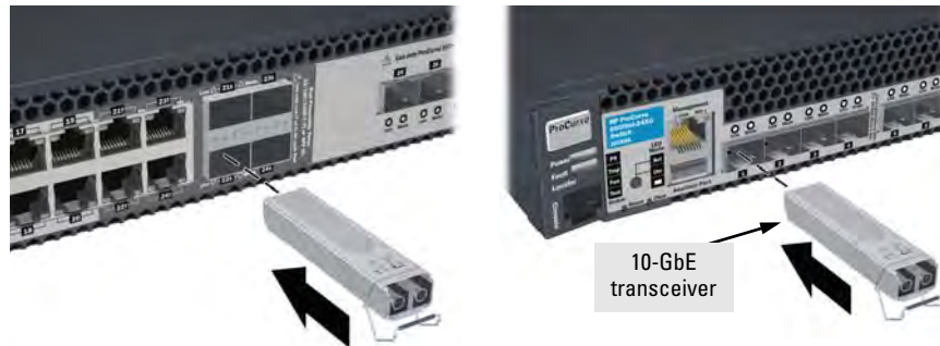
Figure 2-24. Installing a Transceiver
