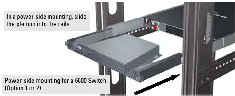
Figure 2-9. Installing an Air Plenum
