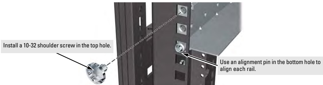
Figure 2-6. Installing Rails in a 4-Post Rack
