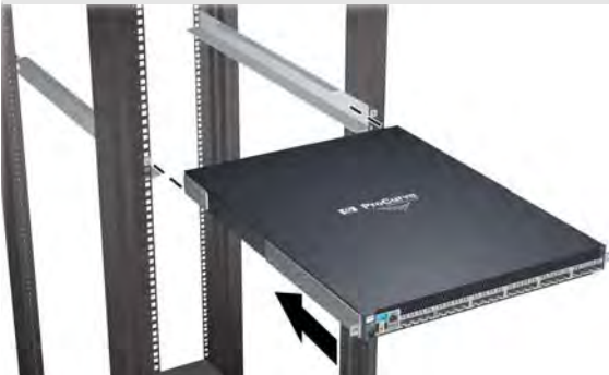
Figure 2-17. Installing a 6600 Switch in a Port-Side HP 10000 Series Mounting
