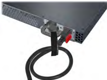
Figure 2-22. Connecting and Securing a Power Cord to a 6600 Switch
