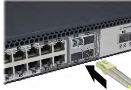
Figure 2-26. Connecting an LC Fiber Optic Connector
