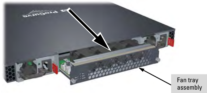
Figure 4-2. Removing the Fan Tray Assembly
