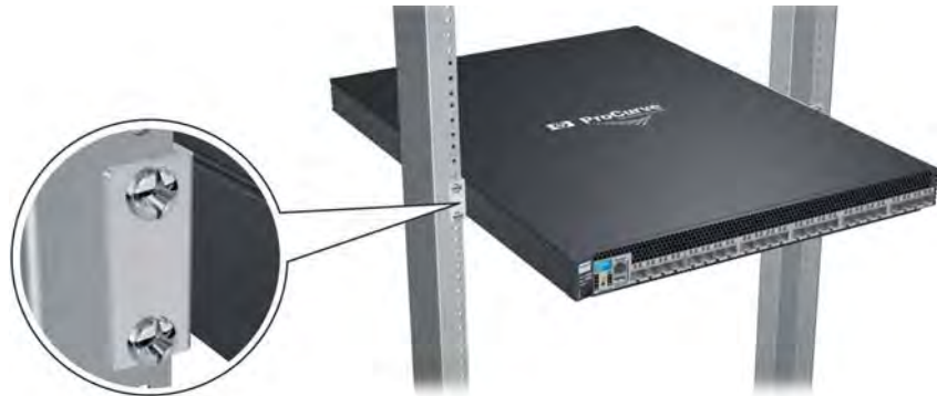
Figure 2-21. Mounting a 6600 Switch in 2-Post Rack
