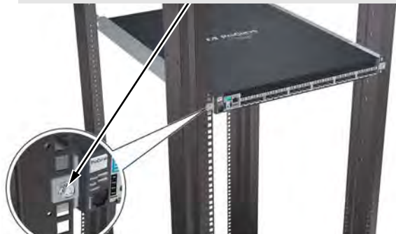
Figure 2-17. Installing a 6600 Switch in a Port-Side HP 10000 Series Mounting
