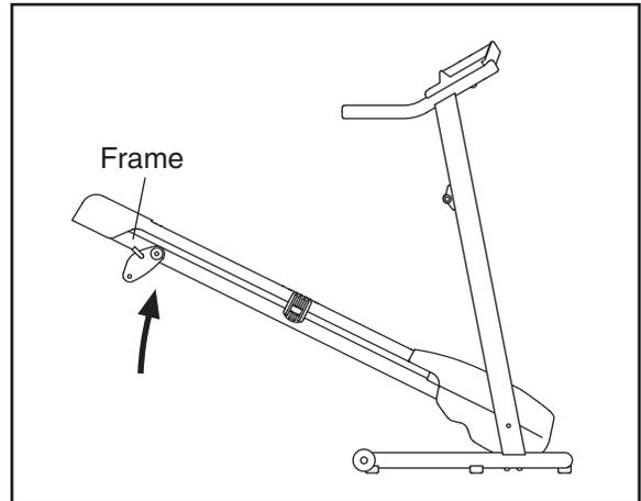
2. Move your right hand to the position shown and hold the treadmill firmly. Using your left hand, pull the latch knob to the left and hold it. Raise the frame until the catch is past the latch pin. Then, slowly release the latch knob; make sure that the catch is resting against the latch pin.
