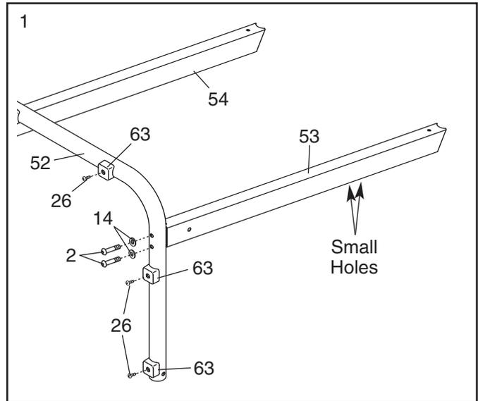
2. With the help of a second person, raise the Uprights (53, 54) so the Base (52) is flat on the floor as shown.
