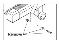
Remove the bolt and washer from the upper end of each handrail. Slide the handrails out of the console housing.
