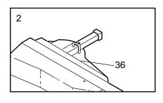
the locked position as shown in drawing 2. Lay the treadmill on its right side. Repeat the procedure for the left Incline Leg. CAUTION: Before using the treadmill, make sure that both Incline Pins (36) are fully inserted at the same height. Do not use the treadmill with the Incline Pins removed.
