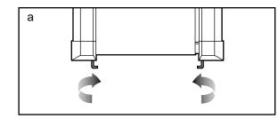
b. If the walking belt has shifted to the right, first remove the SAFEKEY and UNPLUG THE **POWER CORD**. Using the allen wrench, turn the left rear roller adjustment bolt counterclockwise, and the right bolt clockwise, 1/4 of a turn each. Be careful not to overtighten the walking belt. Plug in the power cord, insert the SAFEKEY and run the treadmill for a few minutes. Repeat until the walking belt is centred.
