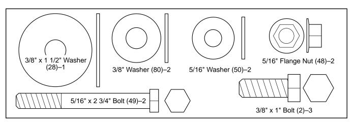
1. Raise the Upright (11) to the vertical position. Insert a 3/8" x 1" Bolt (2), with the 3/8" x 1 1/2" Washer (28), into the lower end of the Upright. Finger tighten the Bolt into the Frame (59).
