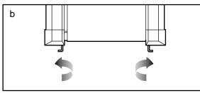
c. If the walking belt slips when walked on, first remove the SAFEKEY and UNPLUG THE **POWER CORD**. Using the allen wrench, turn both rear roller adjustment bolts clockwise, 1/4 of a turn. When the walking belt is correctly tightened, you should be able to lift each side of the walking belt 2" to 3" (5 to 7 cm) cm off the walking platform. The centre of the walking belt should just touch the walking platform. Be careful to keep the walking belt centred. Plug in the power cord, insert the
