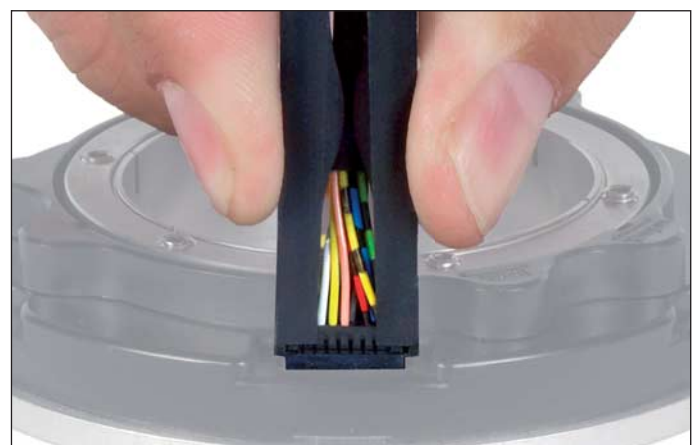
Mounting aid for PCB connector
