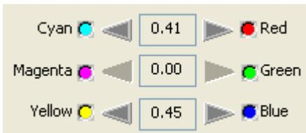
Now save this white balance setting together with the current lamp voltage and filter position on the microscope (if available as an adjustable variable) as an AxioVision hardware setting. This will enable you to achieve reproducible settings for color reproduction. Details on working with hardware settings can be found under this keyword in the AxioVision online help.
