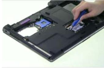
3. Open the LCD module as shown and detach the middle cover carefully.
