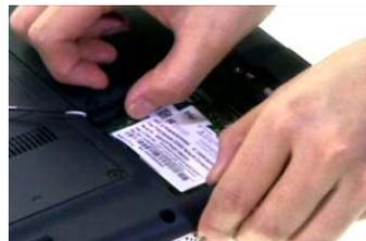
5. Remove the two screws fastening the HDD cover.
