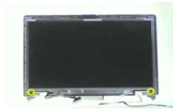
7. Take out the LCD assembly from the LCD panel.
