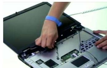
10. Remove two screws holding the LCD module.
