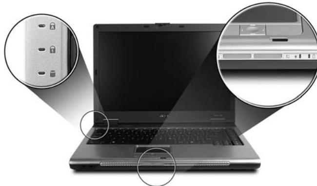
The power, battery and wireless communication status indicators are visible even when the LCD display is closed.
