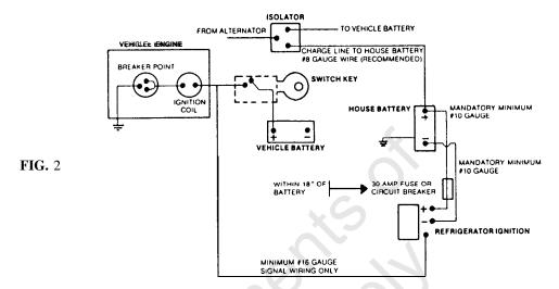
2. The electrical system should also be checked to assure the 12V. DC circuit has been fused; if not, see the following procedure:
