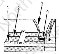
NOTE: The <u>early series</u> only which has the rectangular boiler enclosure, requires that the shield be bent across the middle slightly (I), with a little more angle on the upper tab (2).
