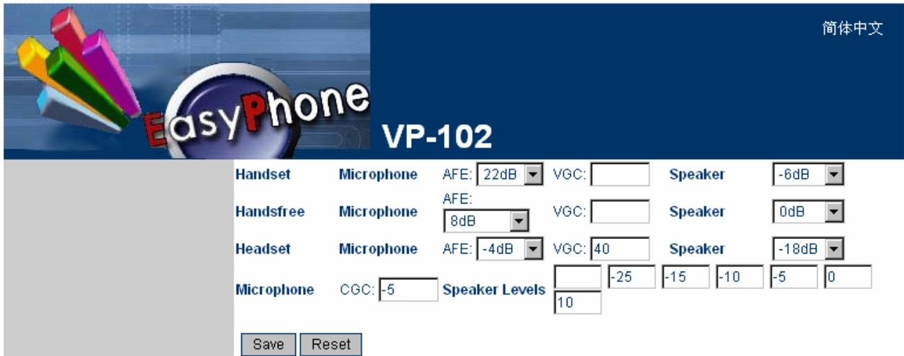
The first 3 rows in the gain settings page shows the 3 modes of operation: Handset, Handsfree, and Headset. Each mode uses the same configuration as shown in the block diagram above. The left hand column (first 3 rows) shows the mode of operation. The various gain settings are described as follows:
