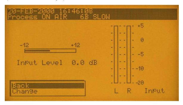
Now, the graphic display of the input level is available. This can be amplified or reduced of 12 dBu. By means of the Jog select a gain in order to have the processor operate around 0 dBm. At the end of the setting, return to Home initial menu.
