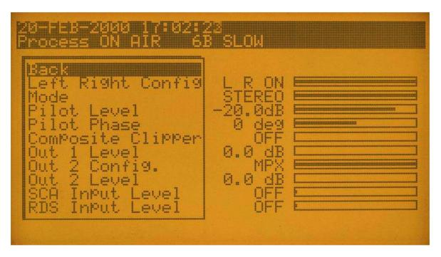
Select the parameter to be changed and carry out the correct set-up by means of the Jog. If you are varying a parameter, but you wish to return to the previously set value, a "X" is shown on the right of the bargraph which not only stresses the control used, but it also goes off if the set value corresponds to the parameter value before any change.
