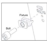
2. Align door handle with fixture and pull the handle down.
