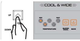
• The temperature values are indicated steplessly from the lowest to the highest temperature.
