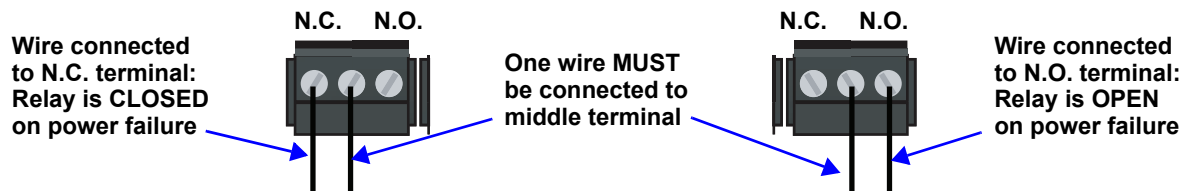
Figure 11 Form C output contact wiring
