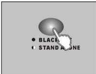
1. Press the **BLACKOUT/STAND ALONE** for 3 seconds, into Stand-Alone mode.
