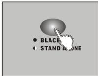
1. Hold on the **BLACKOUT/STAND ALONE** button for 3 seconds to enter Stand-Alone mode.
