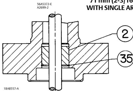
DETAIL OF BAFFLE AND RETAINING RING
