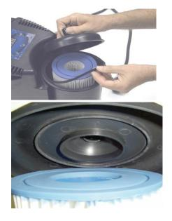
Note: Ensure that the central post and ring on the underside of the cover aligns and fits fully into the top of the filter. Failure to do so may result in water leaks from the filter housing and/or power pack during operation.
