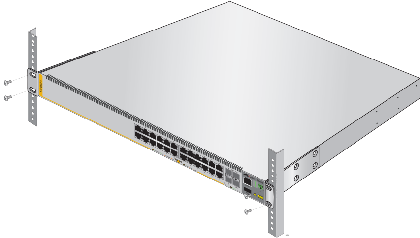
Figure 26. Mounting the Switch Horizontally in an Equipment Rack
