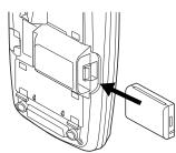
Charge the battery pack for 24 hours. When charging is complete, pull up on the latch to remove the battery pack from the slot. The battery pack in the charging slot also works as an auxiliary power source for the base in case of power failure.
