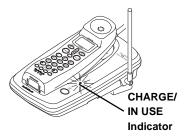
Recharge the battery pack when **Low Battery** flashes on the display.
