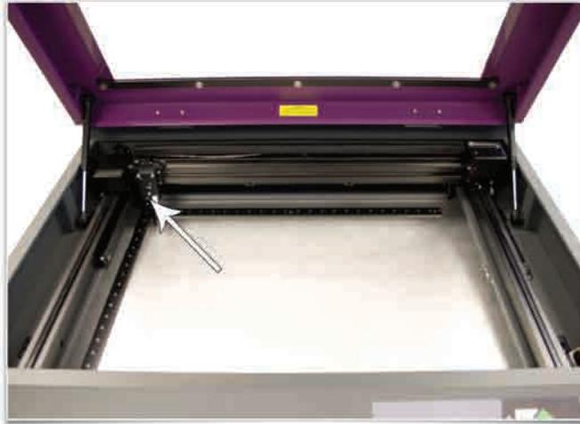
5. Place the focus tool\* against the black lens plate (focus carriage) so that the flat edge of the focus tool rests against the front side of the focus carriage as illustrated. Take note of the fit of the focus tool (it should look like the diagram to the right) in the upper left corner of the system. This corner will be your reference point.
