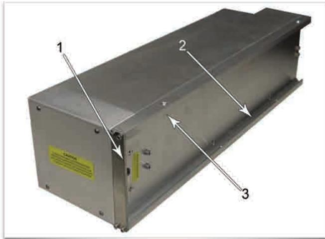
4. Pick up the laser cartridge by the ends and tilt it at a 30 degree angle as shown (1). Mount the cartridge onto the mounting blocks shown in step 2 (page 18) by placing the upper "V" groove on top of the mounting blocks. Slide the cartridge to the right until the outer edge (2) of the alignment plate contacts the inside edge of the large plate of the alignment fork.
