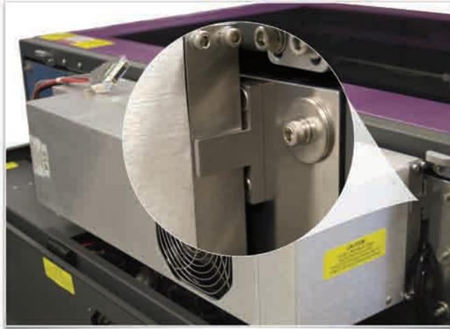
6. Plug in the power connector (1). Close the rear cover, making sure that wires or hoses do not become pinched when the cover is closed. Gently close the rear cover until the sliding latches lock into place.
